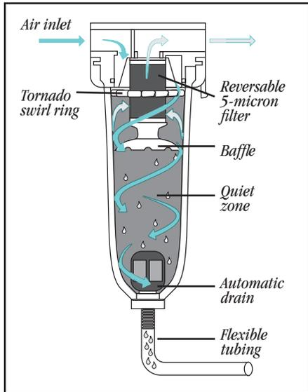
*Tornado-like swirling action removes moisture which collects in the baffled "quiet zone." The reusable 5-micron filter catches smaller impurities. Accumulated liquid is carried away by the automatic drain.*
