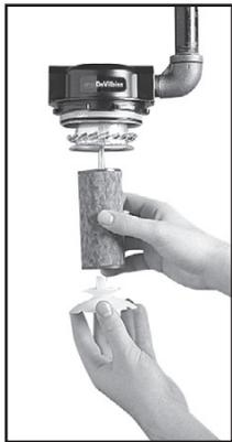
*Quick-release filter bowl and spin-off 5-micron filter element allow one-minute filter changes without tools. Pressure drops are minimized by large air inlet and outlet and large internal air passages.*
